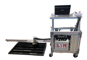
The <u>ScanLIM-2</u> in its optical version, released in 2022, allows the creation of a digital core library that perfectly respects the colors and the scale of all the constituent elements of the cores. In a few clicks, it is possible to view all the cores of a borehole placed end to end.
