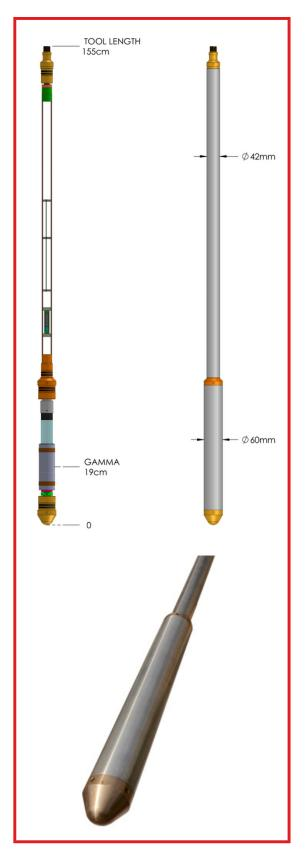
The detector assembly comprises of a 25 x 50 mm (GRS42) or 50 x 150 mm (GRS60) cylindrical Nal crystal coupled to a thermally stabilised photomultiplier tube.
