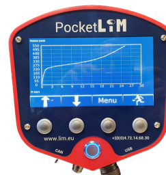
PocketLIM 6G-drilling with smartphone mirroring Pressuremeter curve display NaviLIM application on PocketLIM 6G
