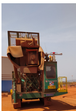
ReichDRILL drill rig with GPS antennas on the cab roof
