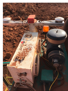
NaviLIM GPS antennas installed on the roof of the drilling rig
