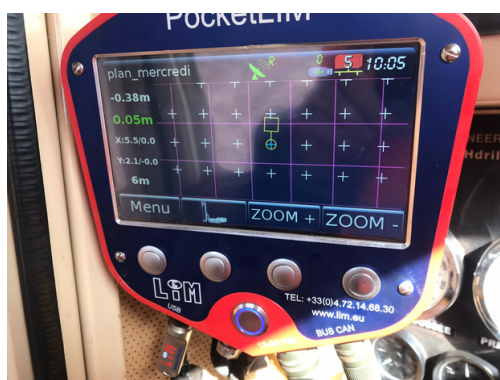
NaviLIM screen with drill pattern and drilling machine
