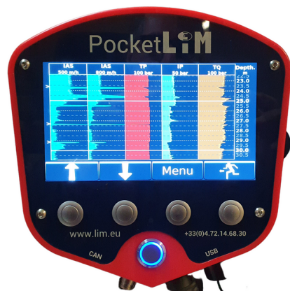
PocketLIM 6G-drilling with smartphone mirroring Pressuremeter curve display NaviLIM application on PocketLIM 6G
