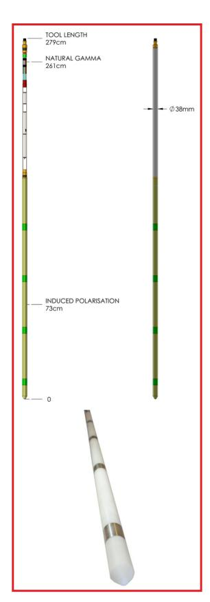
The formations surrounding the borehole are subjected to an alternating square-wave voltage applied via the upper and lower injection electrodes. Following each injection cycle, the resulting potential difference over a section of the formations is analysed as it decays with time. The form of this decay curve is related to the chargeability of the formations.
