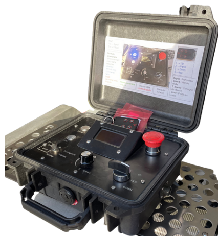
WinchLIM 1200 prototype with its remote control case
