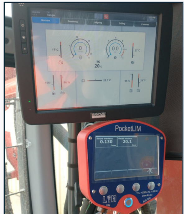
The two TIM™ and PocketLIM systems installed in the Sandvik Ranger™ DX900i drill cabin
