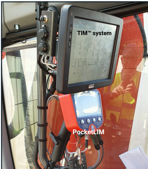
The two TIM™ and PocketLIM systems installed in the Sandvik Ranger™ DX900i drill cabin
