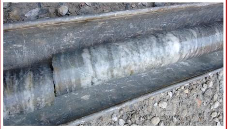
The borehole encountered very hard and abrasive metamorphic rocks (meta-limestones, gneiss with multiple quartz veins and quartz-rich horizons), the photo opposite shows a typical core sample.
