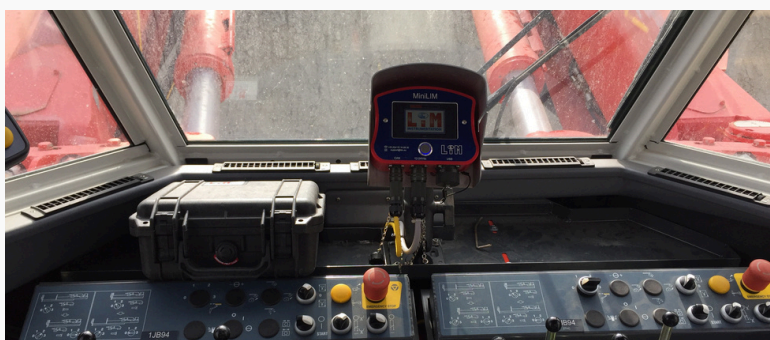
MiniLIM-Drilling installed in the cabin of a drilling machine for underground work (jumbo drill rig)
