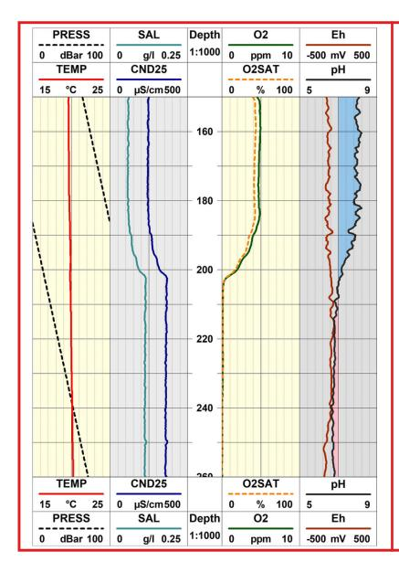
The multi-parameter **WQP48** water quality probe was used to record the example log shown opposite during the geological reconnaissance campaign for the new Lyon – Turin high-speed rail link currently under construction in the Franco-Italian Alps.
