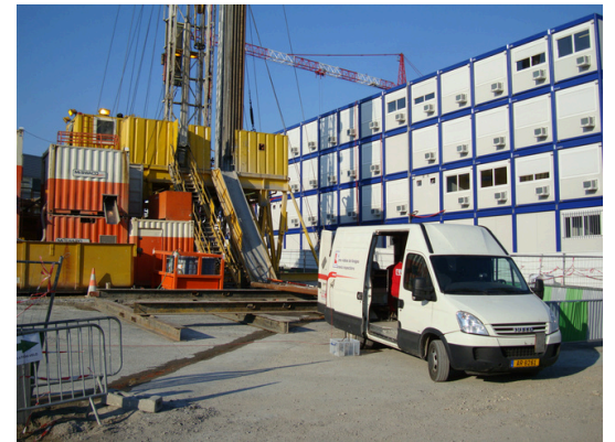
LIM Logging unit on the drill site located in the north-eastern suburbs of Paris
