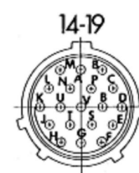
Figure 7: MIL-19 logger connector pin assignments
