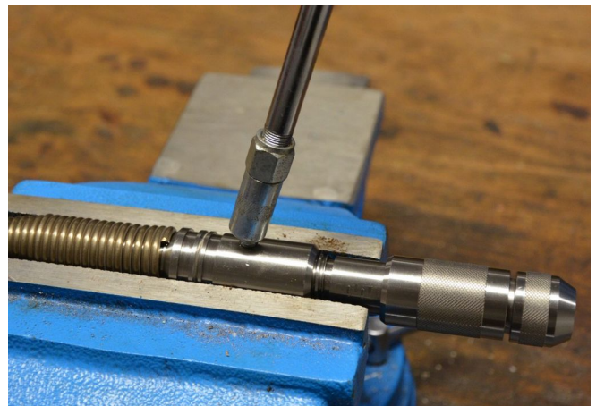
Figure 3: Cablehead greasing in progress
