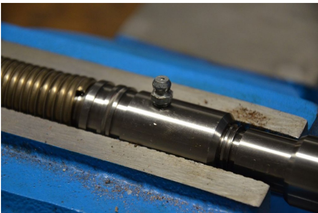
Figure 2: Grease nipple screwed in place in the GO-4 cablehead prior to greasing
