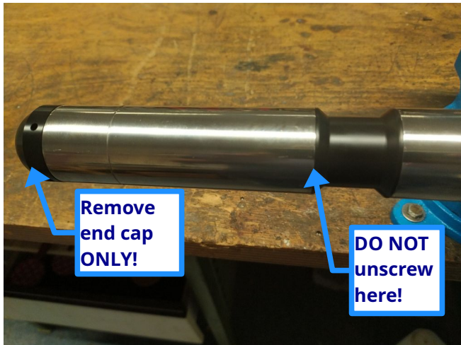
Figure 5: Remove only the probe nose cone to clean the piston
