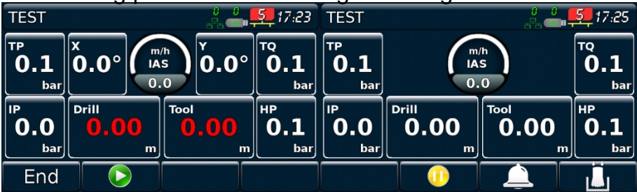
Drilling pause screen Drilling recording screen
