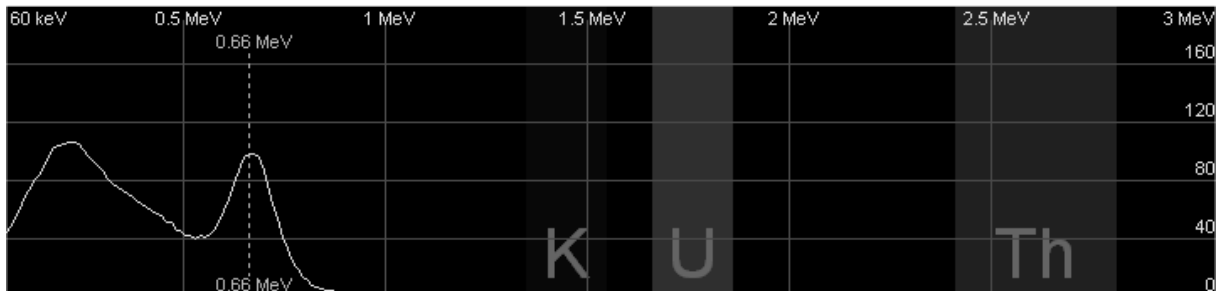
Fig.4.10. Cs-137 calibration source, vertical scale 200 cps
