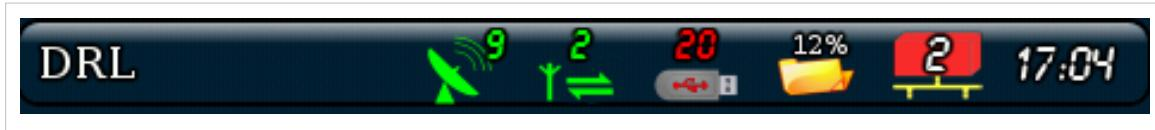
The bar at the top of the screen is always present and informs the operator about the status of the GPS and GSM, the presence of a USB key, the size remaining in the device, the CAN card number on the BUS, and the time. It also gives the name of the drilling currently taking place. This bar also acts as a button that can make the user return to the previous menu when there are multiple applications (choice of the application). The pocketLIM can be described as having two parts:
