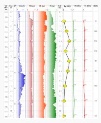
Pressuremeter borehole log
