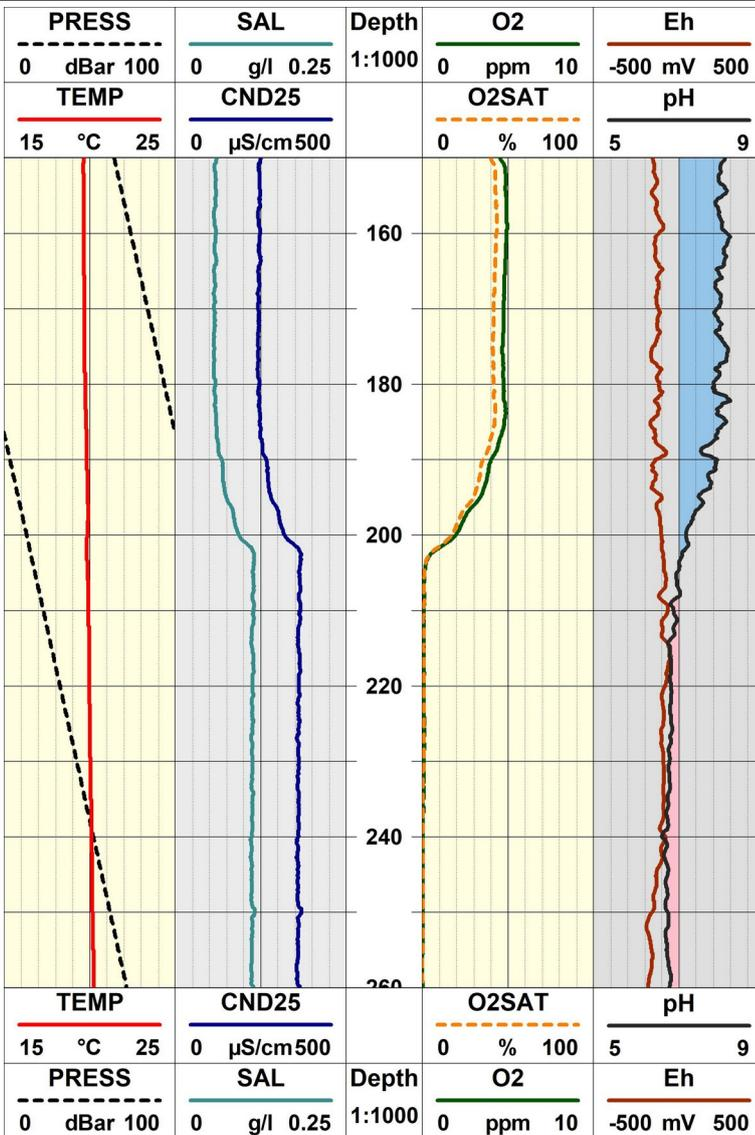
The multi-parameter **WQP48** water quality probe was used to record the example log shown opposite during the geological reconnaissance campaign for the new Lyon – Turin high-speed rail link currently under construction in the Franco-Italian Alps.
